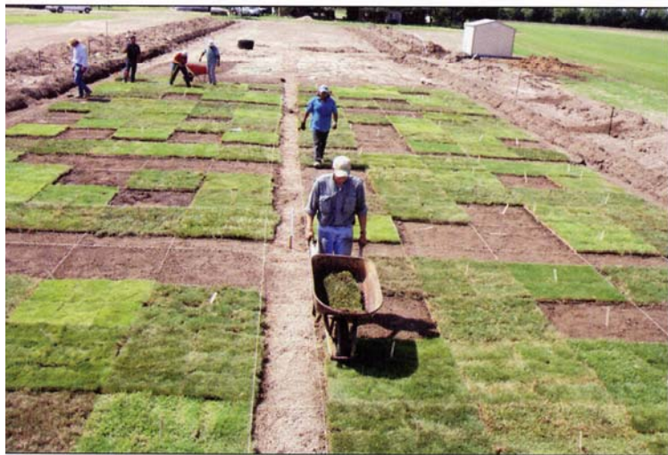
Half of each test plot sample is planted on native soil; the other half is planted on four inches of topsoil which is placed on an impermeable plastic barrier to simulate the SAWS requirement for landscape sod installation—the barrier slopes to drain saturated water flow.
